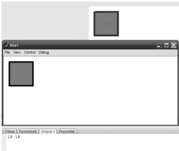
Figure 4-5. The box movieclip on the stage shows its coordinates in the Property inspector. In the SWF, it shows its coordinates in the Output tab, thanks to the trace() function.
