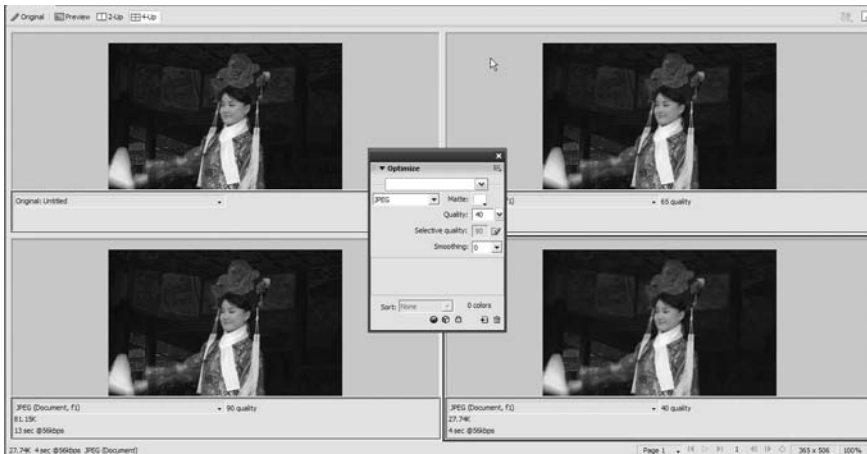
Figure 2-44. 4-Up image optimization in Fireworks CS3 allows you to balance quality against image size.
